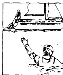
1. Stop boat immediately. Maintain Visual Contact. Deploy Lifesling.
